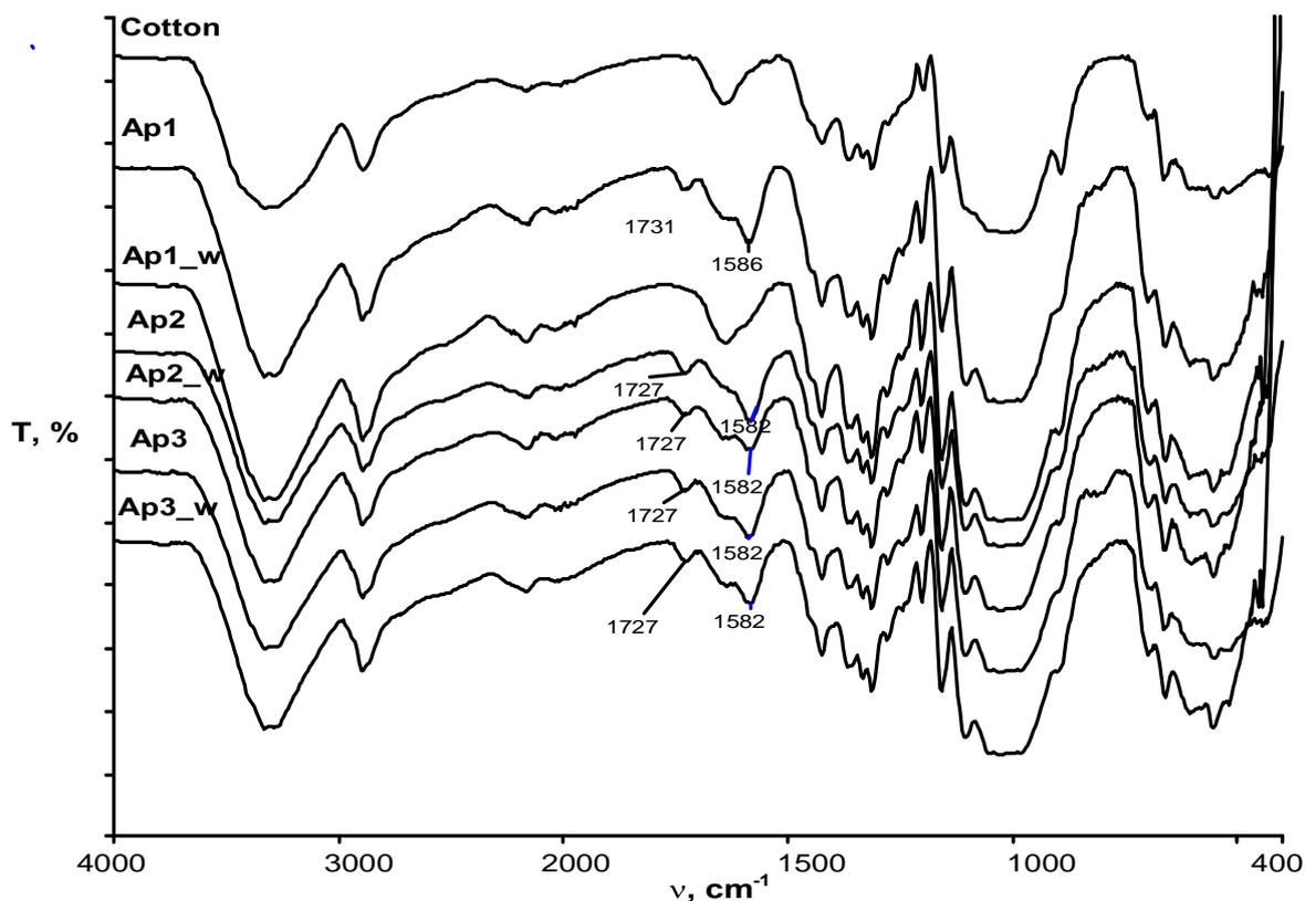
**Figure 3.** FT-IR spectra of cotton and flame retardant cotton fabrics before and after washing cycle
