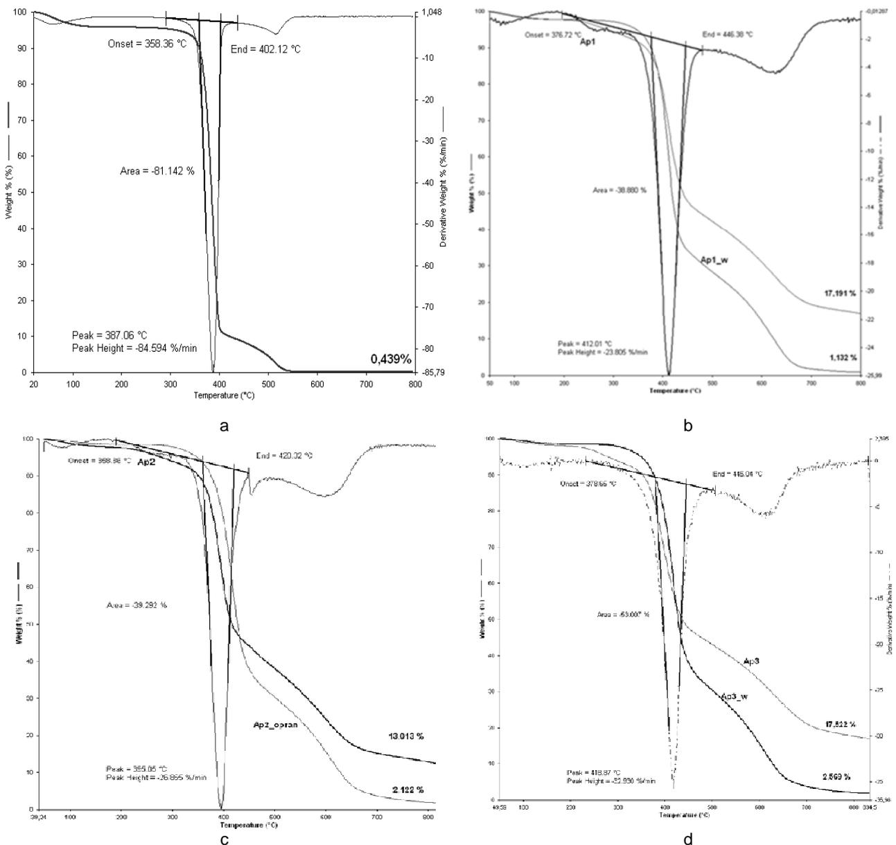
**Figure 1.** TG and DTG curves of fabrics samples: a) cotton, b) Ap1 before and after washing (Ap1\_w), c) Ap2 before and after washing (Ap2\_w), d) Ap3 before and after washing (Ap3\_w), The char residue is given as % of the initial sample weight.
