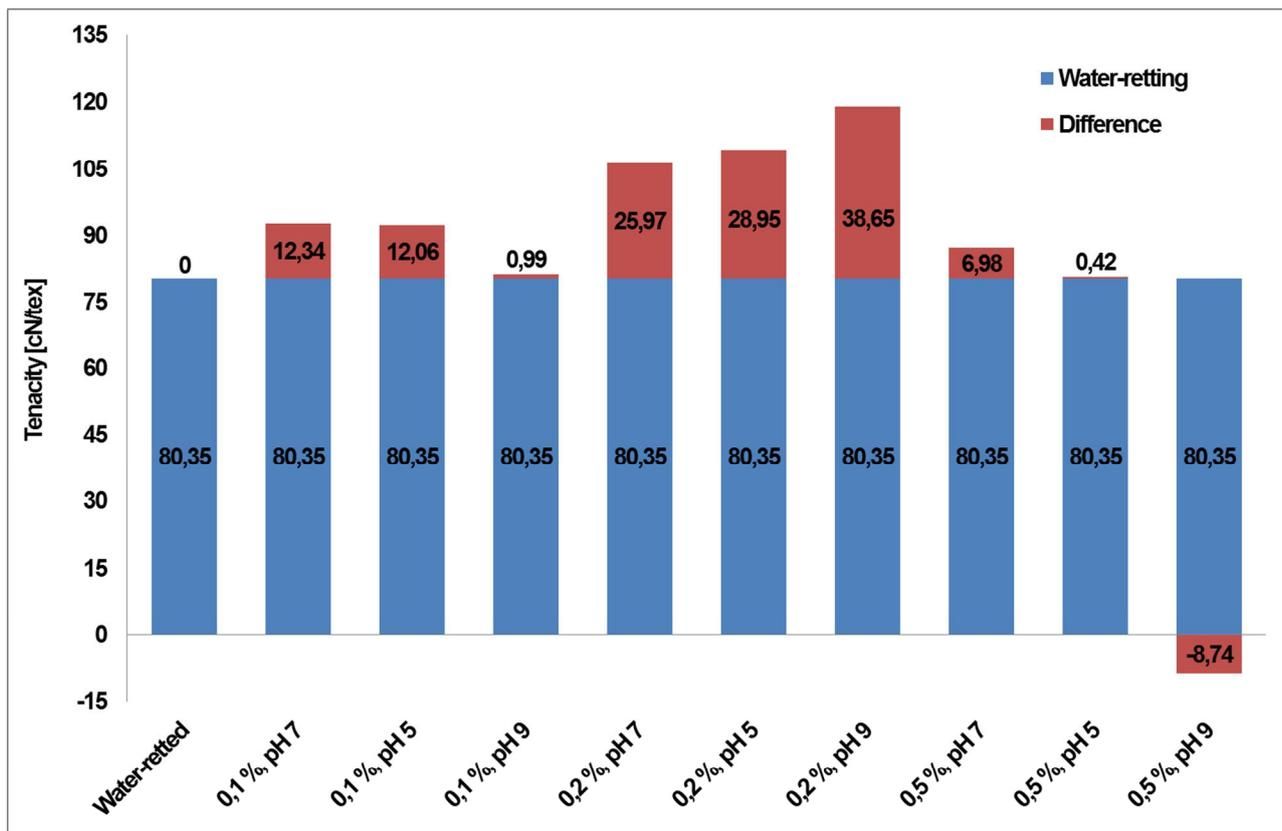
**Figure 3.** The tenacity of flax fibres after enzymatic retting compared to water-retting
